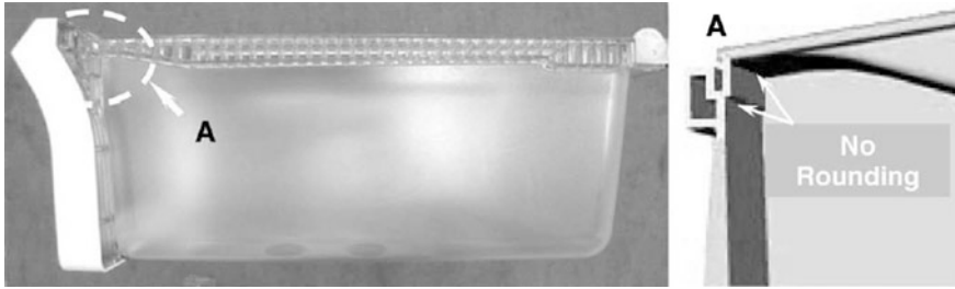
Fig. 9.94 Structure of failing drawer system in field
