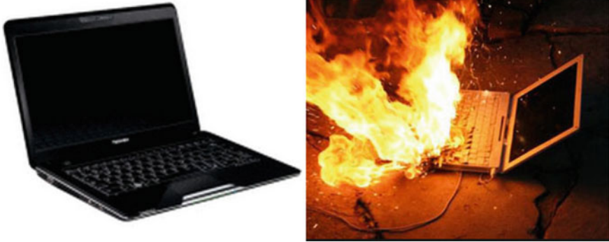
Fig. 2.10 Toshiba Satellite T130 notebook and battery overheating problem
