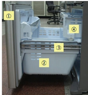
(b) Mechanical parts of the drawer: ① drawer handle, ② drawer, ③ slide rail, and ④ pocket box
